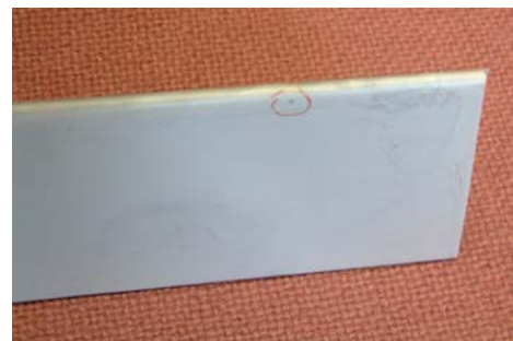
Inclusion on Blade Leading Edge
