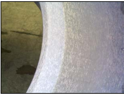
Developed BEA surface showing Titanium grain size and grain flow on a critical rotating aircraft component
