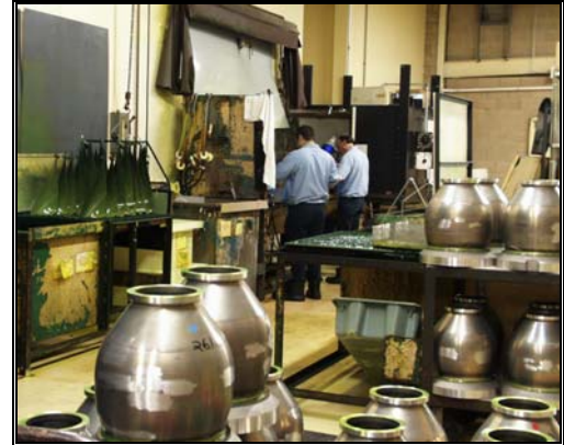
Inspectors in FPI Work Line
