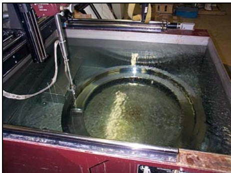
First Generation Upgraded JB Tank doing Turntable Scanning
