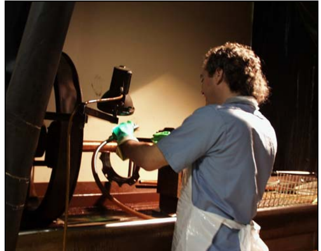
Level II Inspector applying wet fluorescent continuous method on a rod shot (simulation for photo, not under normal UV light conditions)
