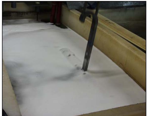
Part on Fixture Submerged Acid Cleaning Solution
