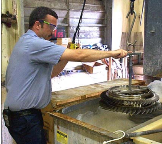
Aircraft Part following Alkaline Cleaning prior to rinse
