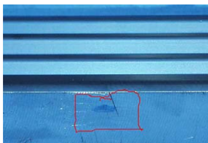
Alpha Indication via Blue Etch Anodize
