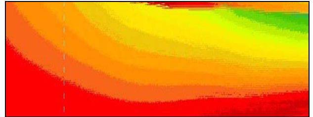
Example of advanced fan blade bondline C-Scan (i.e., top view)
