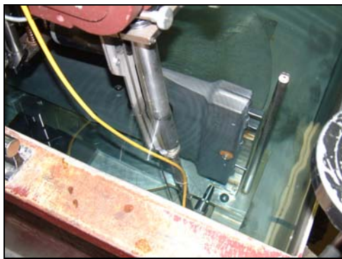
Advanced fan blade in immersion tank - note the beginning of complex geometry at the blade's root stock
