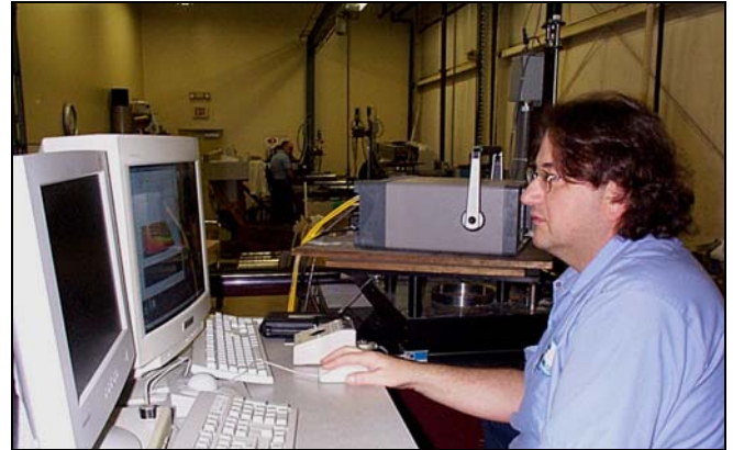
Level III Inspector multi-tasking, analyzing UT C-Scan imaging data while continuing to acquire new data during the same inspection, using our complex contour following motion control immersion tank system
